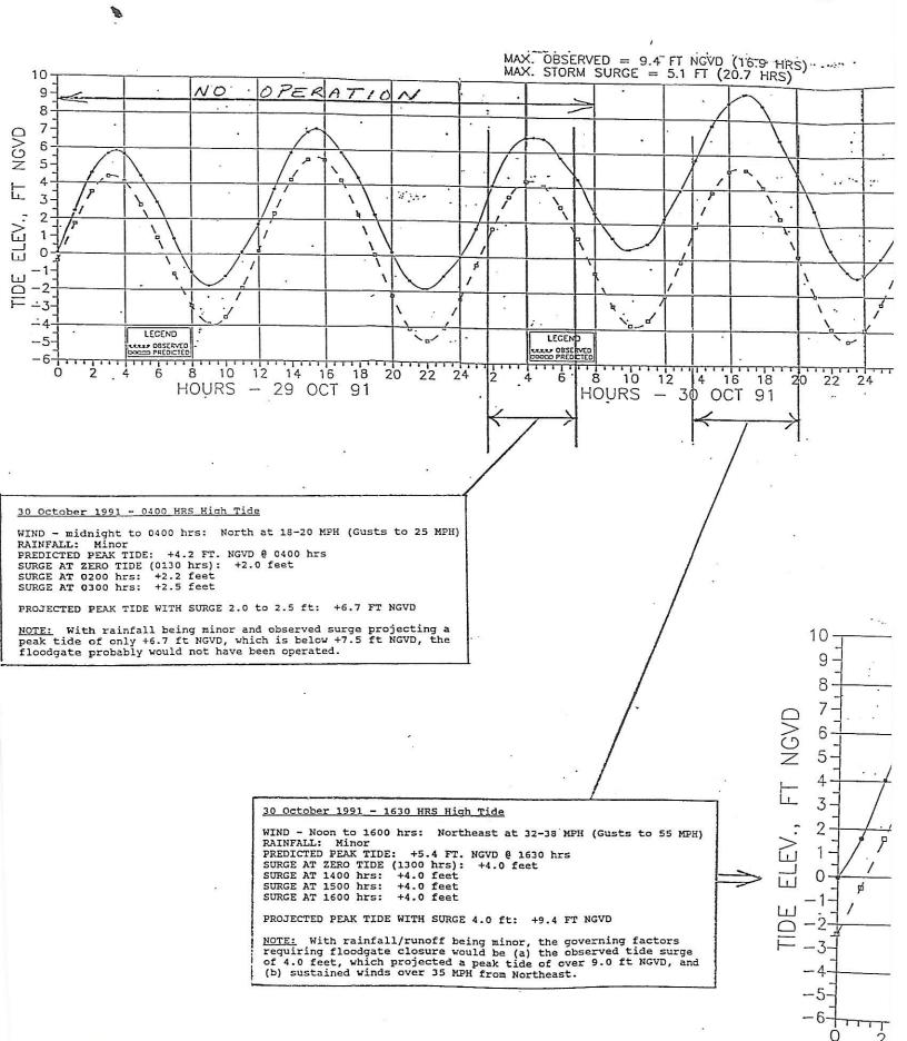
storm and its unpredictable nature, the potential for heavy rainfall, as well as sustained wave overtopping, could not have been ruled out in determining start of gate closure. For the 5 to 6-hour duration floodgates would have been closed, we believe the estuary would have risen no more than 0.2 foot.
